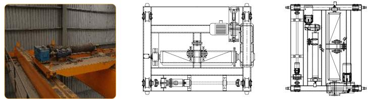
Industrial Crabs can be supplied as standard units or can be custom made. They offer maximum advantages when working in open. These Hoist Crab can have single or twin hoist units as required. The driving arrangement can either be with hand-geared or motor driven type. Micro speed arrangement in hoisting can be provided if required.
